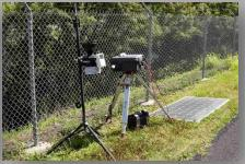
Monitored air quality during fuel tank cleaning ventilation.
