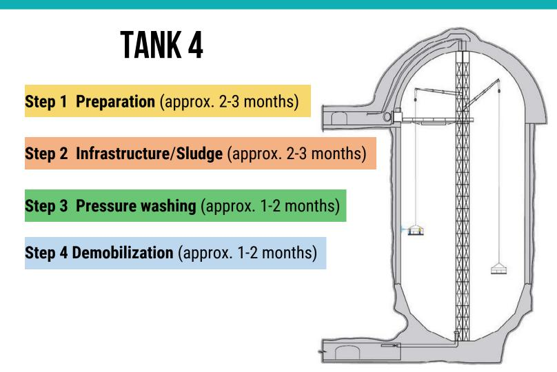
Tank 4 is being prepared for tank ventilation and degassing.
