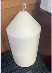
Pipeline "pig" used for cleaning operations
