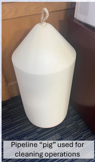
Pipeline “pig” used for cleaning operations
