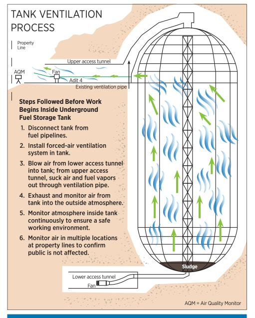
Ventilating large underground fuel storage tanks is a crucial safety measure taken before any cleaning or repair procedure begins. The safety of personnel, the community, and the environment are paramount during this process. Steps for Safe Ventilation of Underground Fuel Storage Tanks at Red Hill Bulk Fuel Storage Facility
