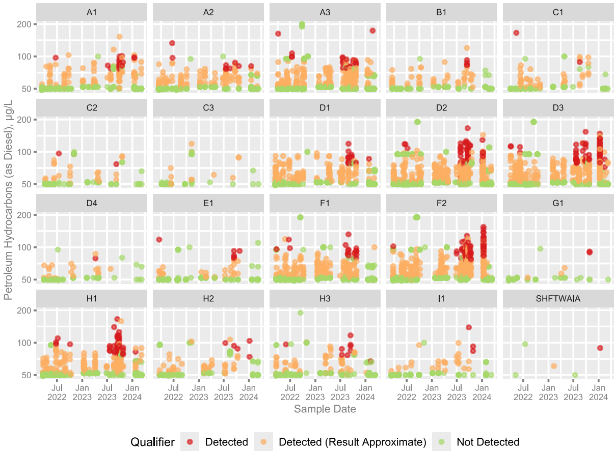
Figure A-2. JBPBH Long Term Monitoring (LTM) TPH-d Data
